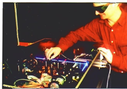
John Girkin and his laser system offers detection of the early stages of tooth decay.
